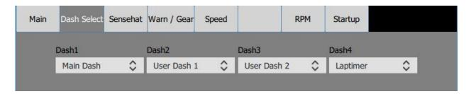
Some dashboards in PowerTune are configurable, such as UserDash. In order to begin building a dash, in the dash select screen, add UserDash1 one of the four active displays. Scroll across to this display, which will be an empty black page. Start building your dash by double tapping the black page. When the main menu is open, all the gauges across all four dashe screens become unlocked and can be moved around. Keep the menu closed when not needed!
