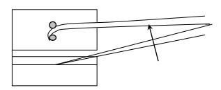
Dress the tip on the Arkansas stone while holding tweezers closed with an O-ring. Draw the point back and forth over the stone while holding the tweezers perpendicular to the motion. The tip can also be dressed by sliding it in the V-groove. It is best to push the tip so it faces into the motion.
