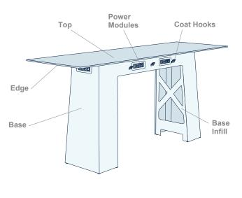
Nimo Bar Finish Section: There are four Nimo Bar components that require finish sections. See izzy+ color card to view color choices for each component. Power module faceplates and coat hooks are the same finish as the base.
