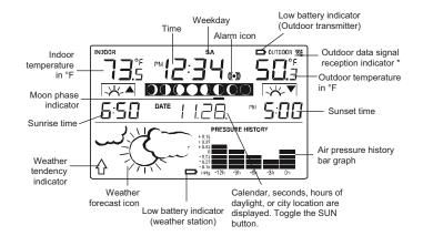
\*When the signal is successfully received by the weather station, the Outdoor reception icon will be flash about every 4 seconds as the temperature updates. (If not successful, the icon will not be shown in LCD).
