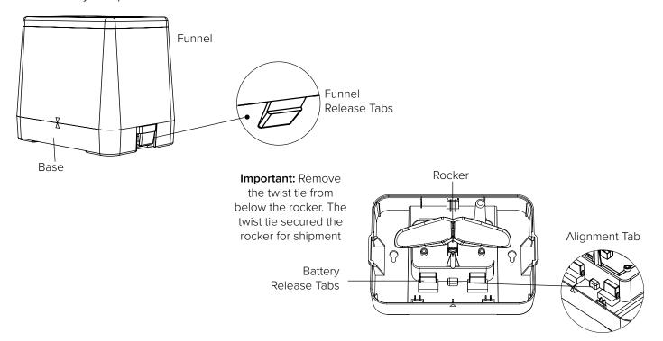
Alignment Tab: An extra piece of plastic used for repositioning the battery compartment correctly. After batteries are installed, make sure this alignment tab is facing the front of the Base to lock all four Battery Release Tabs back into place.
