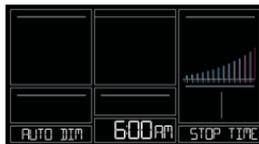
**Note:** If you press the LIGHT button to manually adjust the backlight, the Auto Dim feature will resume at the next scheduled time to dim.
