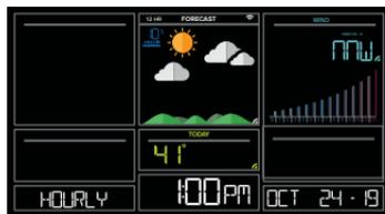
**Note:** If you press the HOUR or DAY button when not connected, station will say CONNECT TO WIFI. If your station is connected, but happens to lose connection with the weather service, it will say WAIT FOR WEATHER when your HOUR or DAY button is pushed.
