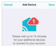
Upon getting the station connected to your Wi-Fi network, the app will explain how your connected sensor should be brought in. Within the next 15 minutes, you should receive an Add Device notification in your app. This is indicated by the Red Cloud and the numbers inside of it. Tap this icon to begin adding your sensor into the app.
