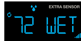
Water Leak Data Example
