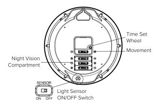
**Note:** The quartz movement will keep the clock running accurately. If the clock does not operate, or steadily loses time, replace the battery.
