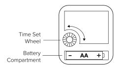
**Note:** The quartz movement will keep the clock running accurately. If the clock does not operate, or steadily loses time, replace the battery.
