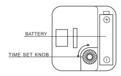
**Battery:** Insert one new AA Alkaline battery according to the polarity marked in the battery compartment.
