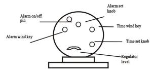
To Set Time: Turn the time set knob to the correct time. Wind the time key fully in the direction the arrow indicates.
