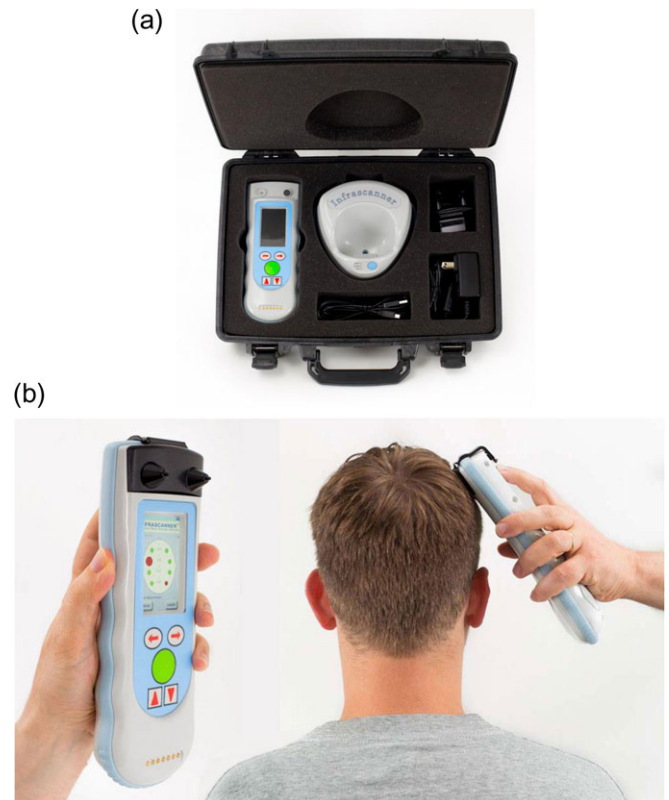
FIGURE 2. Portable NIR detector of intracranial hemorrhage, the Infrascanner: (a) The Infrascanner kit in a ruggedized carry case. (b) The Infrascanner with disposable fiber optic shield in hand and placed on a head.
