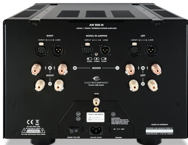
ABOVE: The preamp has two balanced (XLR) and three single-ended (RCA) ins, a line/rec out, and one balanced (XLR) output per side. BELOW: Power amp has switchable stereo/bridged mono inputs with daisy chain outs, all on XLRs. Two sets of 4mm speaker binding posts are offered per channel
