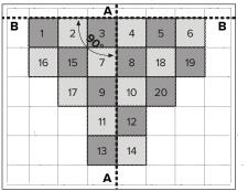
6. Final cuts and completion of the perimeter floor tiles (see clause 3.6) can be done only after you have laid all floor tiles. Ideally, after several hours from the application. When cutting the perimeter floor tiles, allow for a 5 mm gap from any fixed points (e.g. columns, racks and walls). This joint can be pointed with flexible sealant or covered with a strip.
