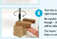
Turn the screwdriver to the right (clockwise) to tighten.
