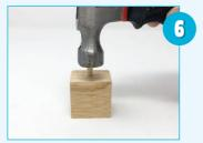
Next, hammer the dowel into the head block.
