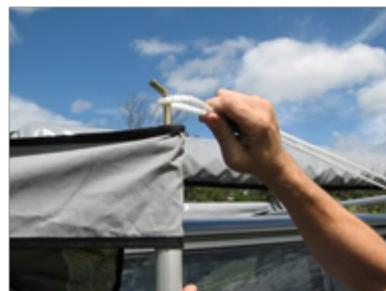
13. Fold out the front awning arm (the arm will be inside the main aluminium track of the awning) Fold the canvas over the arm to expose the plastic end insert, picking up another aluminium bent spigot pole, feed the spigot through the plastic end then fold the canvas over and insert the spigot through the eyelet on the canvas
