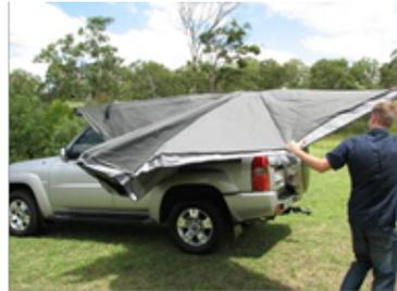
11. Once the SUPA-WING STANDARD is folded out, insert an aluminium bent spigot pole into the arm on the rear of the vehicle, making sure to fold back the canvas to insert the spigot through the plastic end insert on the arm, then fold the canvas over and feed the spigot through the eyelet on the canvas
