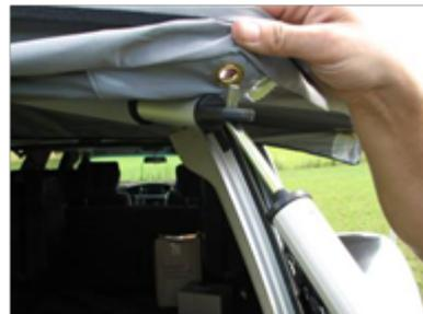
12. Put the strap (the one attached to the roof rack) over the spigot on the rear of the awning and tie off loosely
