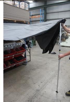
11. Once folded out to the rear of the vehicle, attach the strap to the eye at the end of the rear arm, tighten slightly to bring square off the awning extrusion
