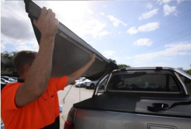
10. Once both wing arms are in position, now swing out the centre arms to support the roof section
