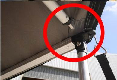
11. Now go along and straighten up the upright poles to your desired height, tighten up the outer tie down straps
