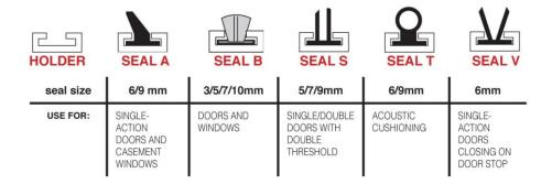
Important – 1-1½mm of the brush or rubber seal is held within the holder. Brush with fin is always ½mm higher than regular brush. Make allowance for this when specifying.
