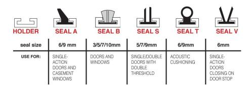
Important – 1-1½mm of the brush or rubber seal is held within the holder. Brush with fin is always ½mm higher than regular brush. Make allowance for this when specifying.
