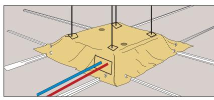
Intumescent card is fixed to the top of the tent to provide entry points for support rods or cables or pipes to pass through.
