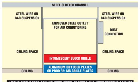
1 HOUR FIRE-RATED CEILING WITH STEEL PLENUM AND INTUMESCENT GRILLES
