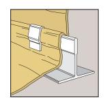
Place the tent over the aircon unit and feed the cable through the ventilation hole, connecting it to the aircon unit according to the manufacturer's instructions. Go to each corner and pull the material away from the fitting over the T-bar and fix the material to the T-bar with the supplied clips. Pinch each clip with a pair of pliers to fix tightly.
