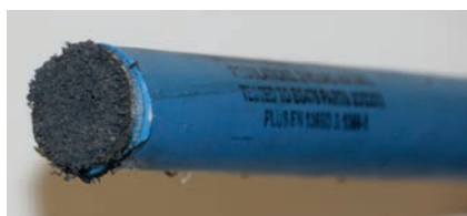
FULLY CLOSED CONDUIT SLEEVE AFTER BEING EXPOSED TO FLAMES
