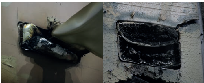
Fireblok® sleeve will crush the PVC ducting, pipe and trunking, completely sealing the opening for over 67 minutes
