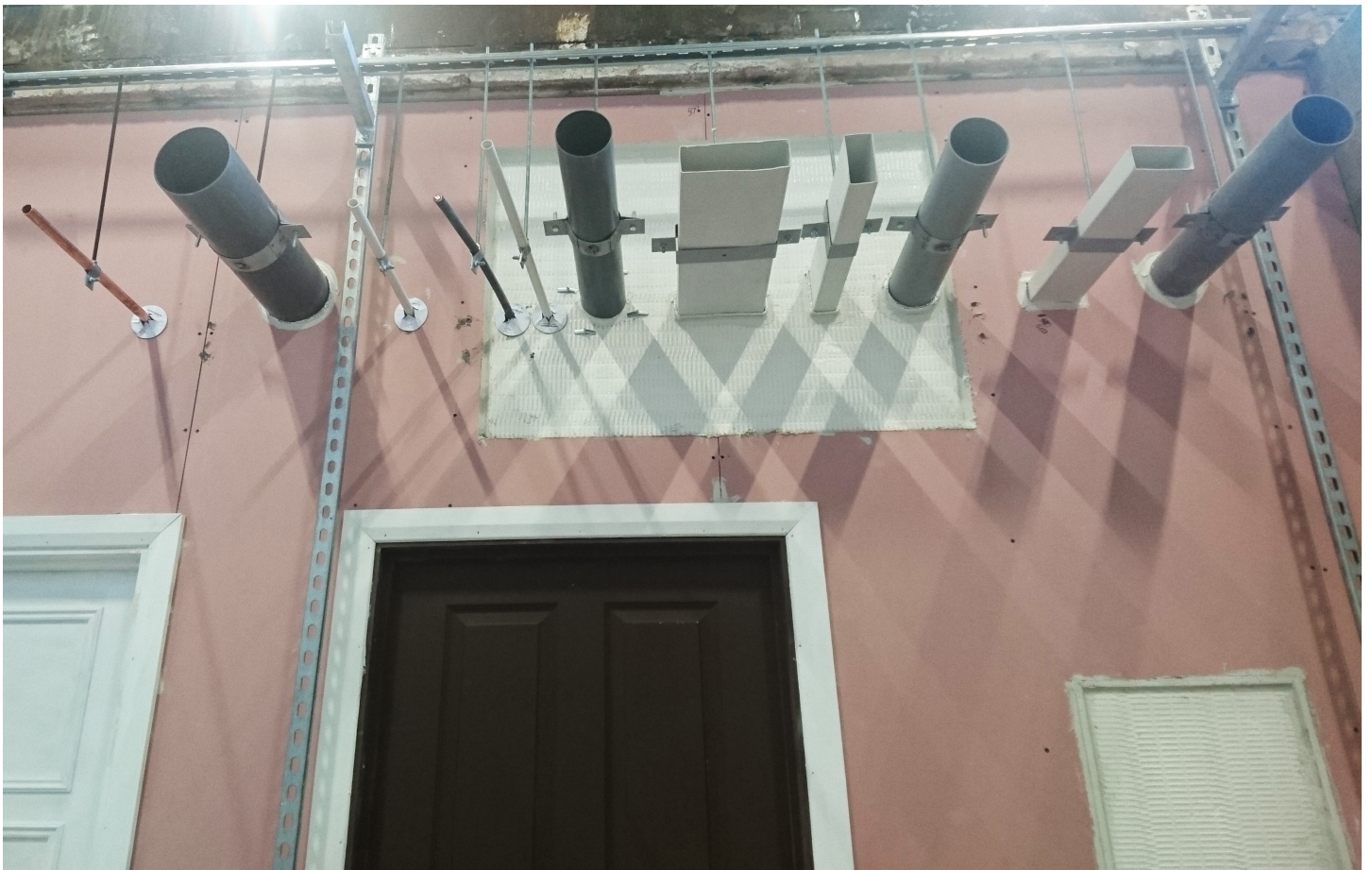
CAG BEING TESTED AT EFACTIS TO EN1366-3 (2009). THE CAG IS AROUND COPPER AND PLASTIC PIPE IN A HOLLOW PLASTERBOARD WALL AND ALSO THE CAG DISC'S ARE ALSO AROUND A CABLE AND A PLASTIC PIPE IN A SLAB WALL. THIS TEST WENT FOR 64 MINUTES.
