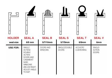
Important – 1-1½mm of the brush or rubber seal is held within the holder. Brush with fin is always ½mm higher than regular brush. Make allowance for this when specifying.
