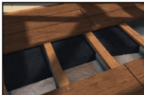
NB: The underfloor fire barrier is supplied to fit a standard 400mm gap between joists, allowing a further 50mm on each side for fixing. Please state if the joist gap differs from 400mm. Skilled tradespeople are required when installing the underfloor fire barrier system. Although the barrier is extremely durable, care must be taken not to tear the barrier during installation. All of the supplied metal plates must be used when fixing the barrier in position.
