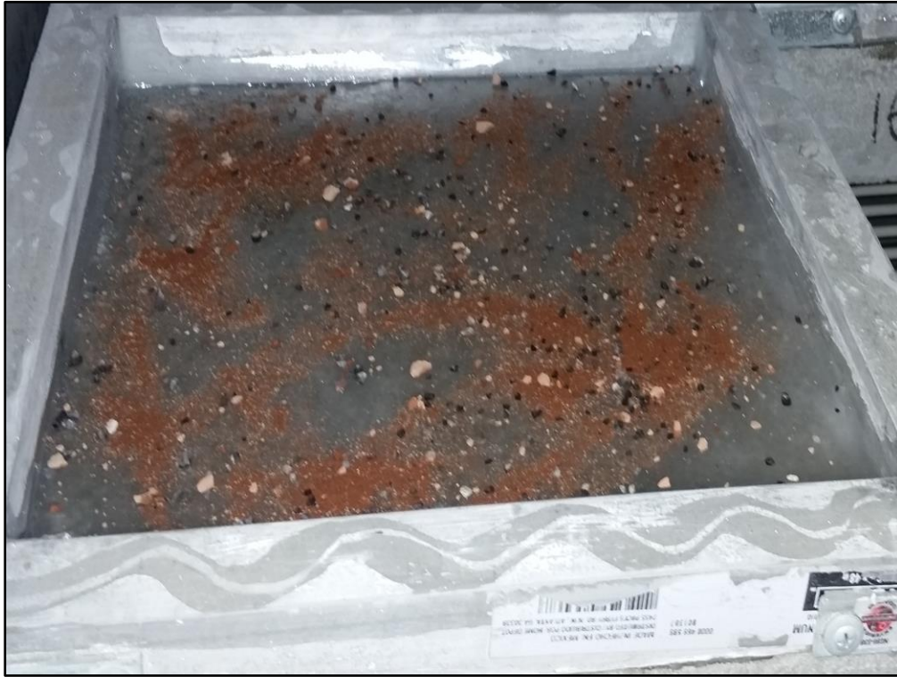
Figure 5. Photo of the Traction Magic sample during testing.
