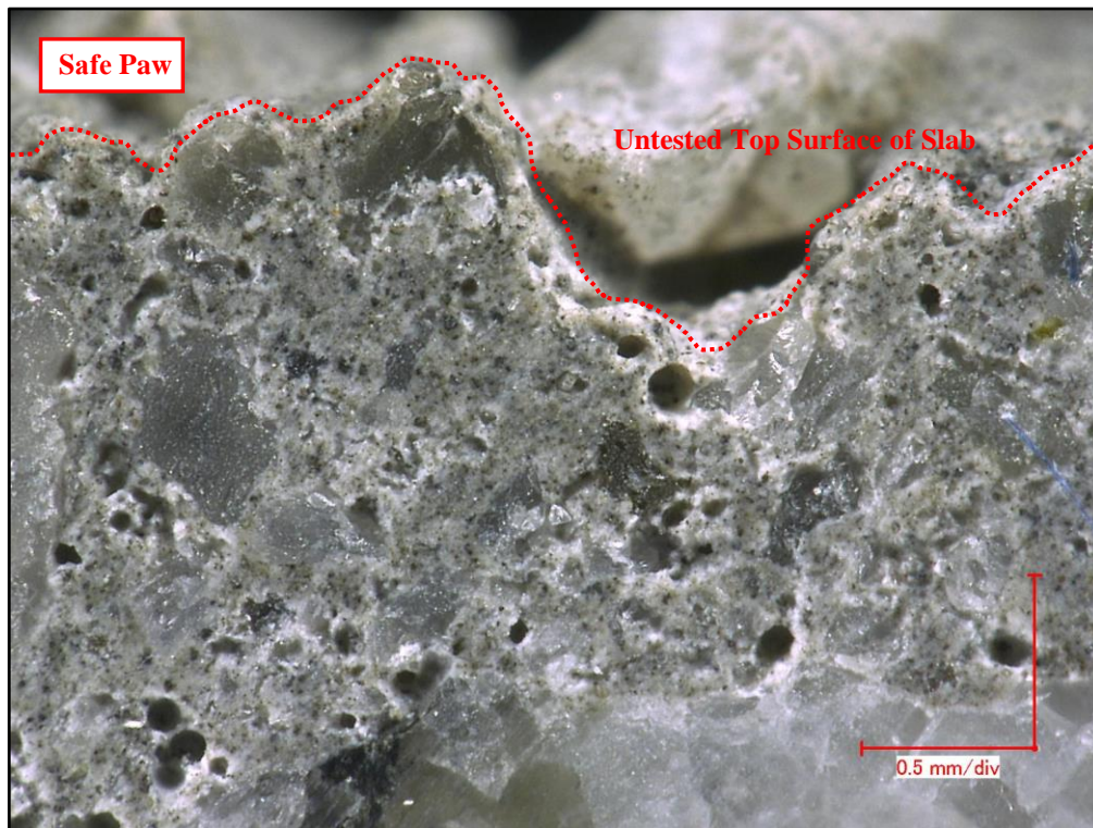
Figure 15. No cracks in concrete beneath the untested top surface (dotted red line) of the Safe Paw test slab. No relatively darker paste is present beneath top surface.
