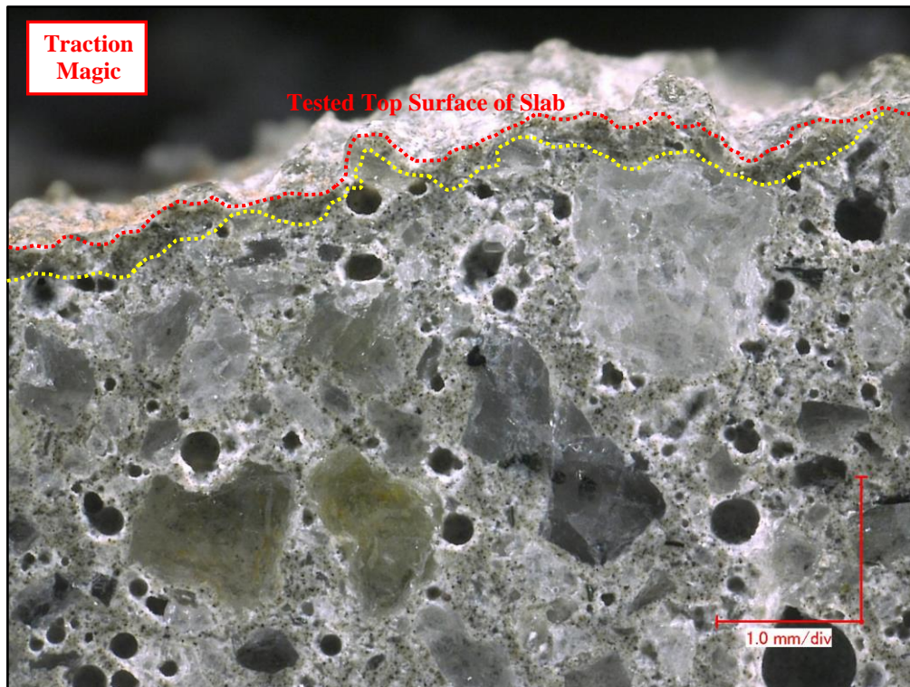
Figure 12. No cracks in concrete beneath the tested top surface (dotted red line) of the Traction Magic test slab. The yellow dotted line is the approximate absorption depth of the salt scaling solution.
