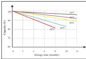
Note 2: The above curves are based on laboratory testing data @  $25^{\circ}\text{C}\ 40\%\text{RH}.$
