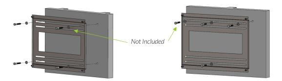
STEP 2: Make sure the Keyhole on the inverter aligns with the 3/8-16 stud on the wall mount bracket. Secure the Inverter on the wall mount bracket with  $4 \times 3/8-16$  Serrated flange locknut (included with wall bracket).
