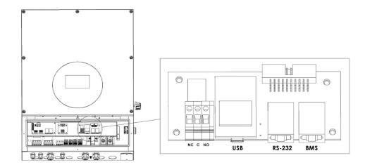
The inverter is equipped with several communication ports for alternative communication interfaces in order to communicate with a PC with corresponding software. Follow below procedure to connect communication wiring and install the software.
