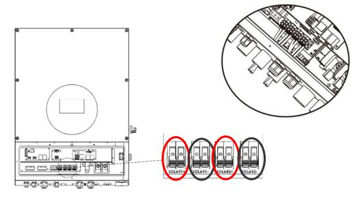
**Step 5:** Tie in your EPO or RSD button to the RSD terminals. Once PV is connected and all polarity verified, turn the PV Disconnect switch on the side of the inverter to the "ON" position. Once the inverter is up and running test your rapid shutdown procedure and verify it is functioning properly.
