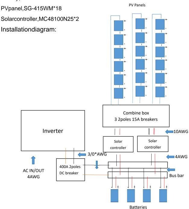
For the 300A 2poles DC breaker and wire could be smaller according to the load. Amp=power of load(w)/50(V), based on the amp, the DC breaker and wire can be choosed.
