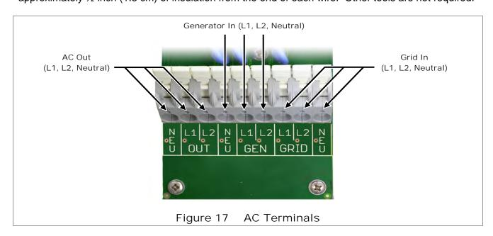
The terminals labeled **L1** and **L2 GRID** are used to connect to the two utility grid "hot" wires. The **L1** and **L2** wires are usually black and red respectively, and read 120 Vac each when measured with respect to neutral. In a standard service, **L1** and **L2** are 180 degrees out of phase and should read 240 Vac when measured from one to the other.
