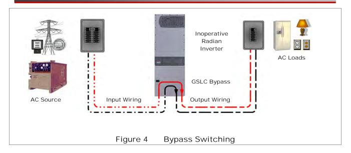
Both manual and automatic double-throw bypass switches are commonly available in a range of sizes and options. These are highly recommended for systems with more than a single inverter.
