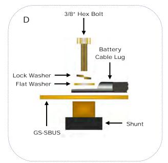
Figure 16 DC Cable Hardware (Radian inverter)
