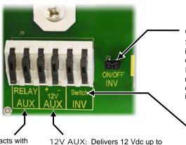
ON/OFF INV JUMPER (J3): Overrides the SWITCH INV terminals when installed. When installed, the inverter is On. The On or Off states can then only be controlled by the system display. NOTE: J3 is installed to the **ON** position during manufacture, but the Radian inverter is given an external **OFF** command at the same time. Its initial state will be Off.
