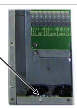
Figure 14 Chassis Ground TBB
