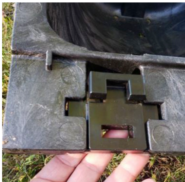
Figures 10. and 11. Close-ups of slot for sliding retainer clip
