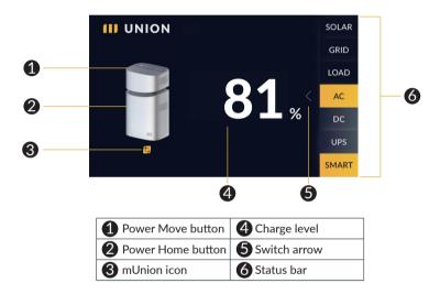
After tapping the **1** or **2**, you can separately read the Power Move's or Power Home's charge level through the pages shown below:
