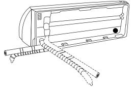
3. Use scissors to cut down the length of the insulating sleeve to reveal about 6 in (15 cm) of the refrigerant piping. This serves two purposes:
