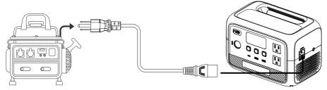
**Note:** Make sure your generator delivers the AC output with charging voltage, frequency, and Grid Self-adaption Mode voltage that meet AC2P's specifications.
