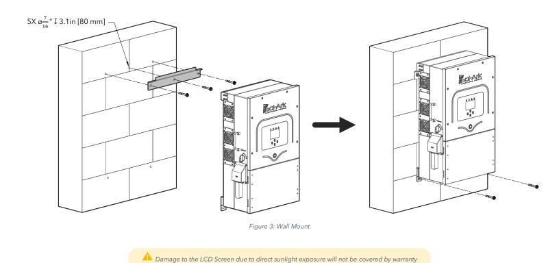
H. Mount the inverter in the optimal orientation as shown below.
