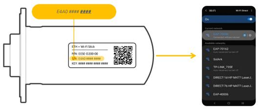
Figure 41: E4A0-#### serial number and EAP network
