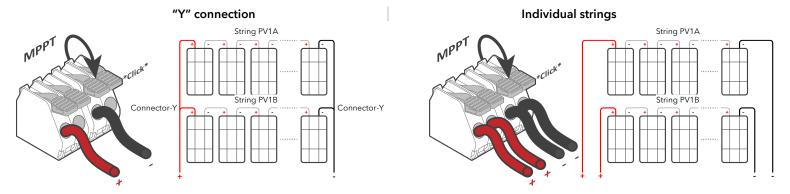
Figure 9: MPPT wiring and PV connections
