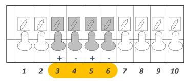
Figure 17: CT input pins on inverter
