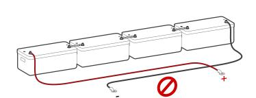
**A** DO NOT reverse polarity. The system will be damaged, and warranty will be voided!
