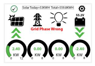
Figure 37: Grid phase wrong error
