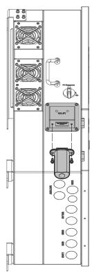
Figure 40: Connecting Wi-Fi dongle to Sol-Ark 12K-2P-N
