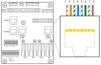
Figure 33: RJ-45 port configuration
