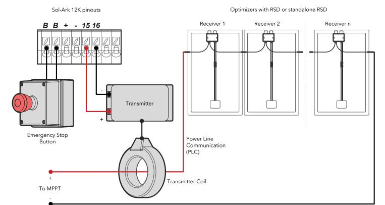
Figure 19: Emergency stop and RSD installation
