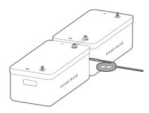
Figure 13: Temperature sensor for Lead-Acid batteries
