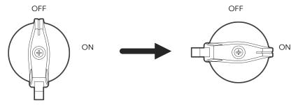
Figure 20: Built-in PV DC disconnect
