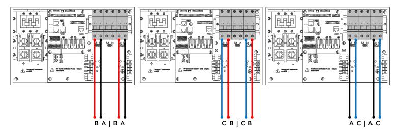
Figure 38: Example of correct phase sequence
