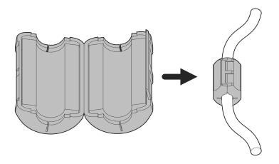
a) Installation of small suppressor on appliance power cord
