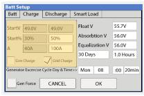
Figure 11: Generator and grid charge settings
