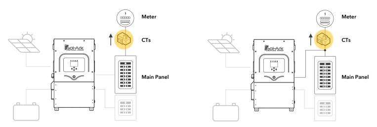
Figure 16: Installation of CTs for a) back-feed breaker and b) line side tap
