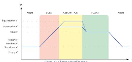
Figure 32: Charge controller curve
