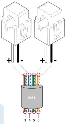
Figure 18: CT wire extensions with shielded CAT 6 cable
