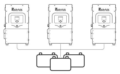
Figure 7: Single battery bank for parallel inverters
