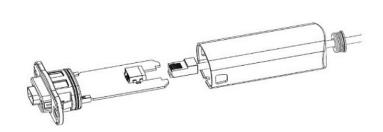
Figure 39: Connecting Wi-Fi dongle to ethernet
