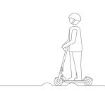
Do not pass the deceleration strip, elevator threshold, cobbly road and other irregular roads in high speed. Keep middle or low speed (5-10km/h) when driving on rugged road. Bend your knees slightly for better adjusting the complex roads mentioned above
