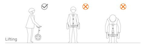
For your safety, motor power is cut off when the miniPRO is lifted off the ground in Balance Mode. When the miniPRO is put back down it will begin balancing again. Do not lift the miniPRO by the fenders or mainframe; you risk pinching or injuring your fingers/hands. Please lift via the knee control bar as shown above.
