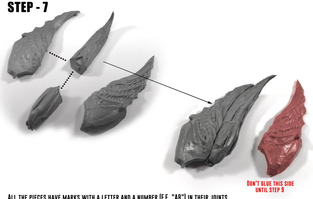
ALL THE PIECES HAVE MARKS WITH A LETTER AND A NUMBER (F.E. "A8") IN THEIR JOINTS. Connect every piece with the one that has the same mark, as shown in the picture.
