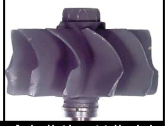
Impact damage caused by foreign material entering the turbine housing or compressor housing is clearly visible on the turbine wheel or impeller.
