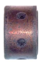
Bearing damage due to hot shutdown
