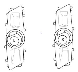
The right-side pedal has a right-hand thread (removes counterclockwise, installs clockwise); the left side pedal has a left-hand thread (removes clockwise, installs counterclockwise).
