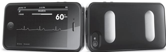
Figure 1: AliveCor Heart Monitor (AliveCor Inc.).
