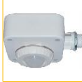
PIR sensor 120-277Vac input, IP65 rating, max detect height is 15m.
