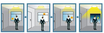
The lamp lights on 100% illumination or dims to maintain the preset illumination level against ambient light.
