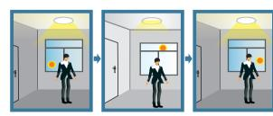
The lamp lights on 100% illumination or dims to maintain the preset illumination level against ambient light.
