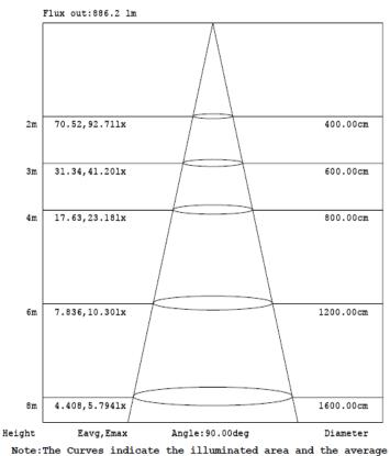
illumination when the luminaire is at different distance.
