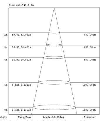
Note: The Curves indicate the illuminated area and the average illumination when the luminaire is at different distance.
