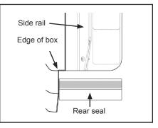
B. Mark seal leg and then cut notch in seal.
