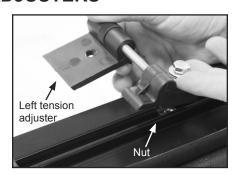
B. Turn 1-1/4" bolt with flat washer onto nut in front bar. Leave loose for now. Repeat for tension adjuster (marked "R") on passenger side of cover and leave bolt loose as well.
