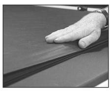
E. For additional protection, manual Slide Lock are located under rear bar on passenger side. Push Slide Lock to engage; pull to disengage.
