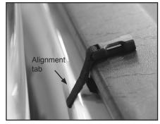
C. Slide left tension adjuster until it engages under side rail (see Step 5F). Push bar back and forth to line up holes. Do not turn adjustment wheel. Insert bolt from top and nut from bottom.
