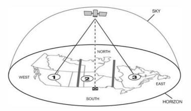
Figure 10: SIRIUS Antenna Pointing Guidelines, Canada
