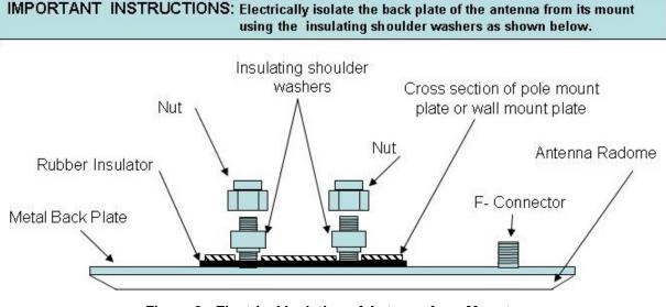
Figure 8: Electrical Isolation of Antenna from Mount
