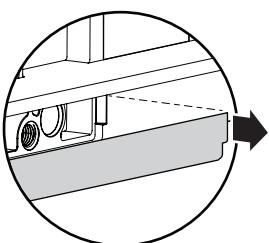
If cover is accidentally installed, pry cover with screwdriver.
